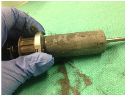
Figure 6.1: The problem of thickening in MRF-based clutch.
