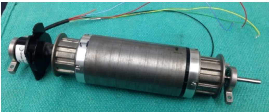
Figure 4.3: The developed armature-based MRF clutch
